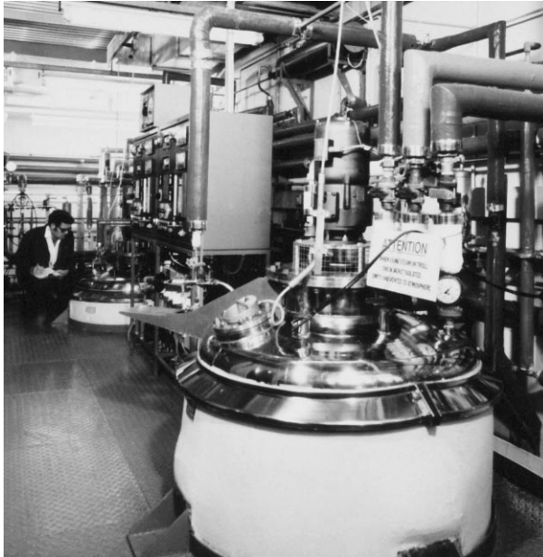
Figure 11: Industrial-scale equipment for the manufacture of FMD vaccine, c. 1966.
